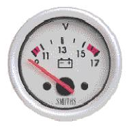
This antique voltmeter has a safe zone of 10.5 to 15.5 volts. Outside that is the danger zone.
